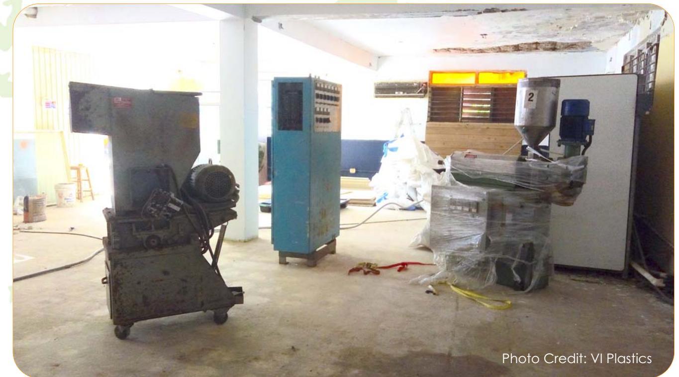
Shredder to shred the discarded plastic & Extruder to form the plastic
