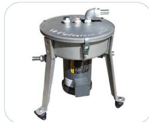
Biofuel Equipment to clean used vegetable oil
