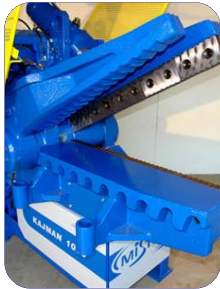
Alligator Shears to cut up metal
