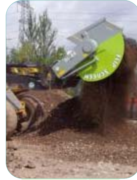
Flipscreen to process glass aggregate and organics
